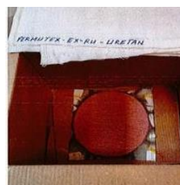
Fig. 1: Textile samples with Cu deposition by DC/RF Magnetron Sputtering Impregnated with ITOBINDER-AG-Acrylate Impregnated with PERMUTEX-EX-RU-Urethane
