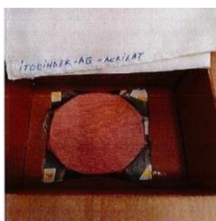
Fig. 1: Textile samples with Cu deposition by DC/RF Magnetron Sputtering Impregnated with ITOBINDER-AG-Acrylate Impregnated with PERMUTEX-EX-RU-Urethane
